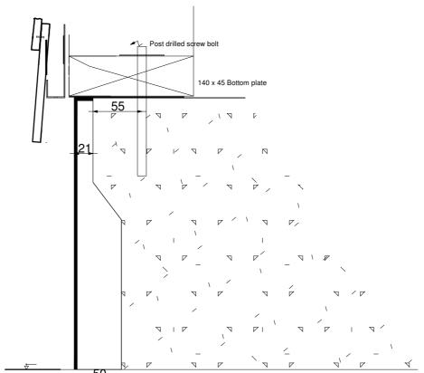
140 x 45 timber framed wall post drilled screw bolt EPS foam
