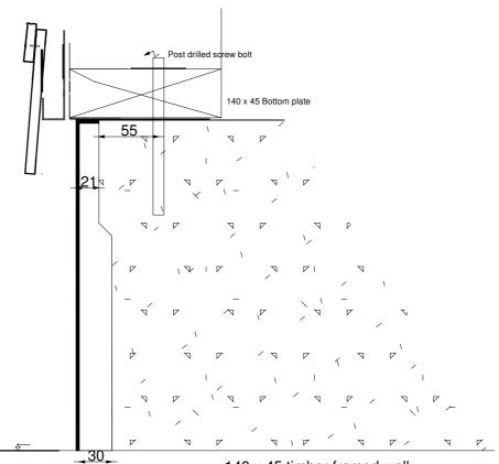
140 x 45 timber framed wall post drilled screw bolt XPS foam
